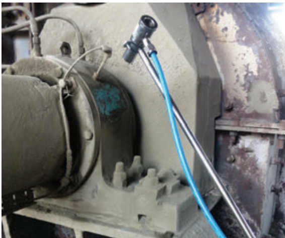
Fig 8: Bearing housing cooling by energy efficient device (Arrest Master ABS)
