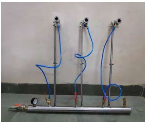
Fig 09: Kiln Shell cooling by Energy efficient device (Arrest Master ABS)
