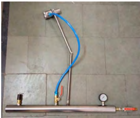
Fig 08: Bearing housing cooling by Energy efficient device (Arrest Master ABS)
